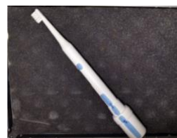
Figure 3. The electric toothbrush is connected to a brush extension that contains a movement sensor.
