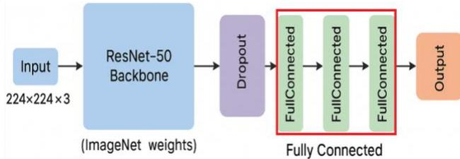
FIGURE 1. CNN Architecture for Binary Classification of Pick Body Presence
