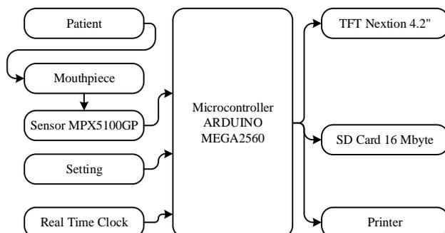
FIGURE 1. The Block Diagram of Peak Flow Meter
