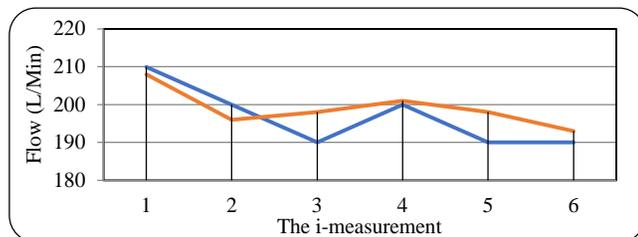
FIGURE 3. Result of Measurement Of Flow Value At A Pressure 0,7 Kg/Cm<sup>2</sup>. (The orange line indicates the design and the blue line indicates the standard unit)
